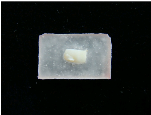
Figure 1 The tooth sample was mounted in the resin with an area of 2 mm × 2 mm.
