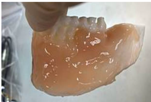
Figure 3 Soft tissue reconstruction on a 3D-printed mandibular model. Food-grade silicone (Shore 20A) was manually applied to the surface of the 3D-printed mandible model to simulate gingival and soft tissue morphology.
